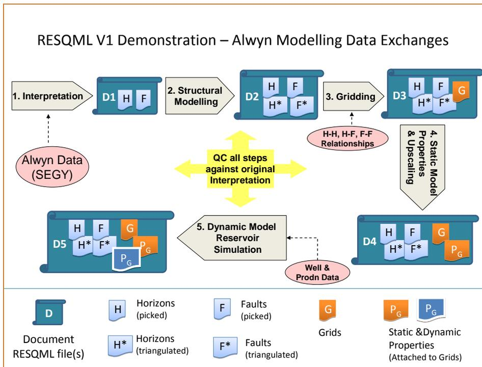
Figure 6 RESQML data exchange by multiple parties/software packages using Alwyn field data set.
