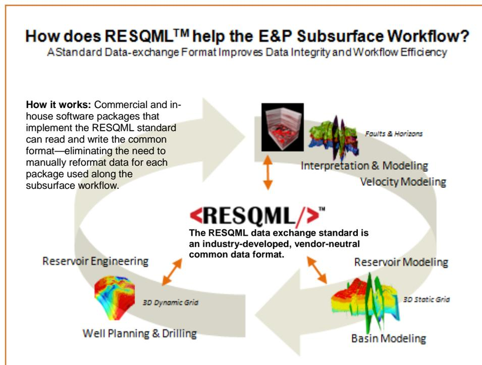
**Figure 1 Implementing RESQML in software used in the E&P subsurface workflows streamlines data flow between the many software packages used, improves efficiency in those workflows, and ensures data integrity. This figure shows workflows supported by the current version of RESQML.**
