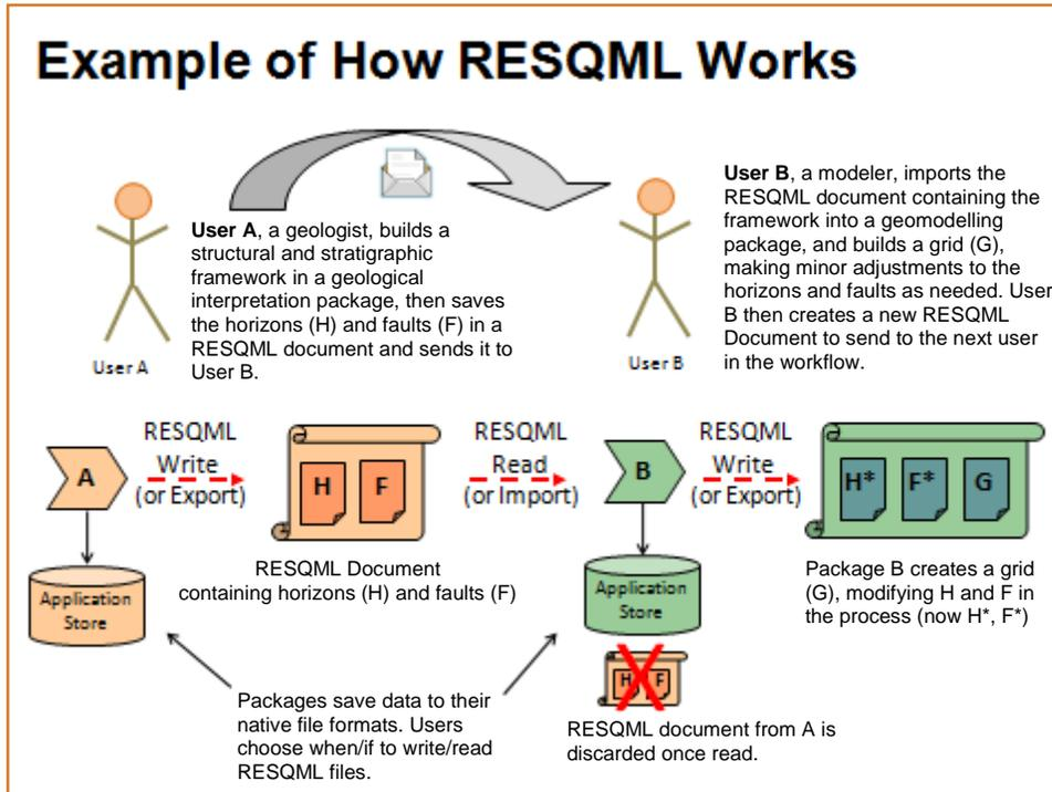
Figure 7 A user writes (exports) a file to the RESQML format, which may be read (imported) by the next software package in the workflow.
